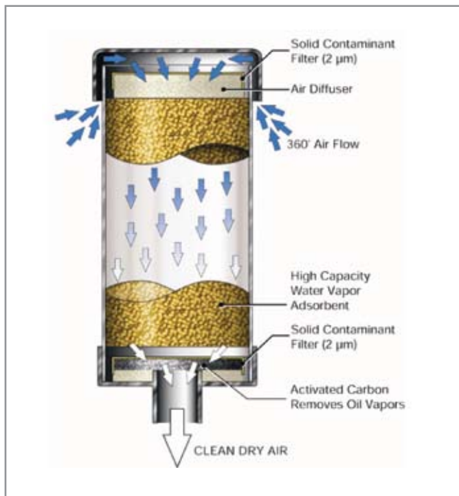
Figure 4 | Desiccant elements can be used to arrest airborne contaminant ingress at a relatively low cost. (Courtesy of Trico Corp.)
