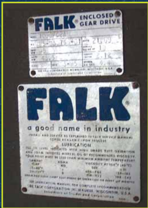
Figure 11. Gear drive faceplate label showing viscosity parameters
